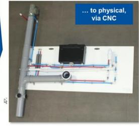
5. This digital model generates manufacturing details automatically, from a parametric bill of materials, which in turn generates code for DXF files for our CNC machines
