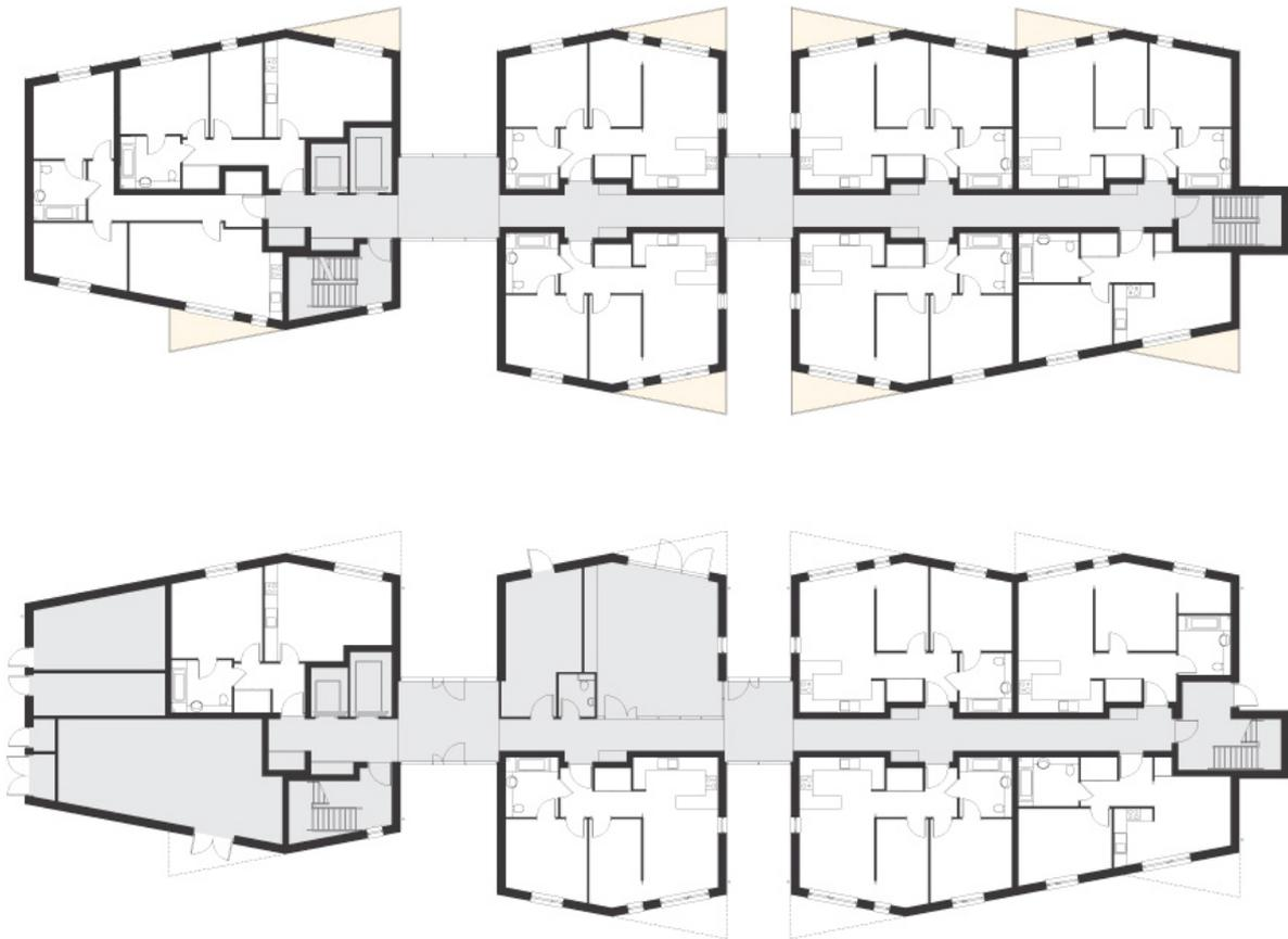
*Bruyn's Court typical floor plan (top) and ground floor plan (bottom)*
