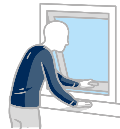
Figure 7. Windows should have easily-operated controls between 750mm and 1200mm from floor level.
