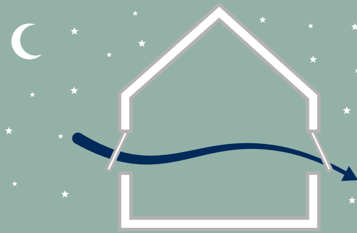
Figure 2. During hot weather, it is often best to open the windows of a Passivhaus at night only, in order to exclude warm air during the day.
