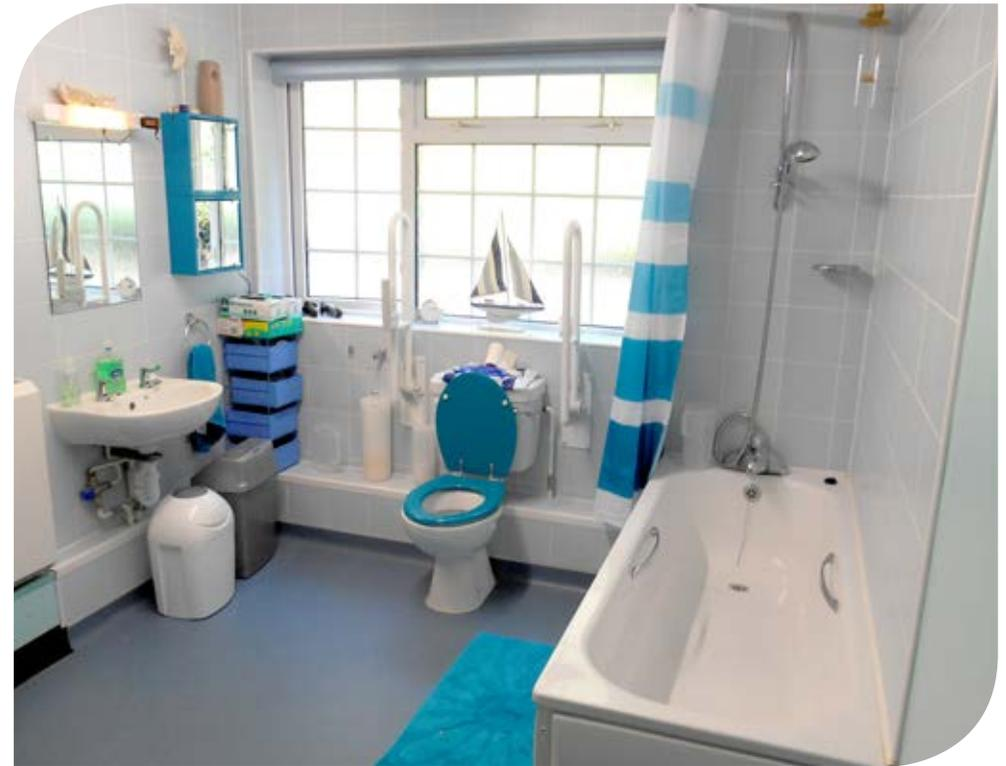
**The photograph displays a bathroom in a supported housing scheme for people with learning disabilities and sight loss. The finishes of the flooring, tiles, toilet seat and grab rails have been chosen to ensure the bathroom is fully contrasted and highlight the difference between key adjacent surfaces.**
