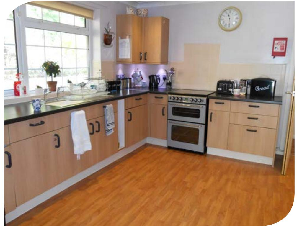
**The photograph displays a kitchen in a supported housing scheme for people with learning disabilities and sight loss. The finishes of the kitchen units, plinth, worktop, tiles and sockets have been chosen to ensure the kitchen is fully contrasted and highlight the difference between key adjacent surfaces.**
