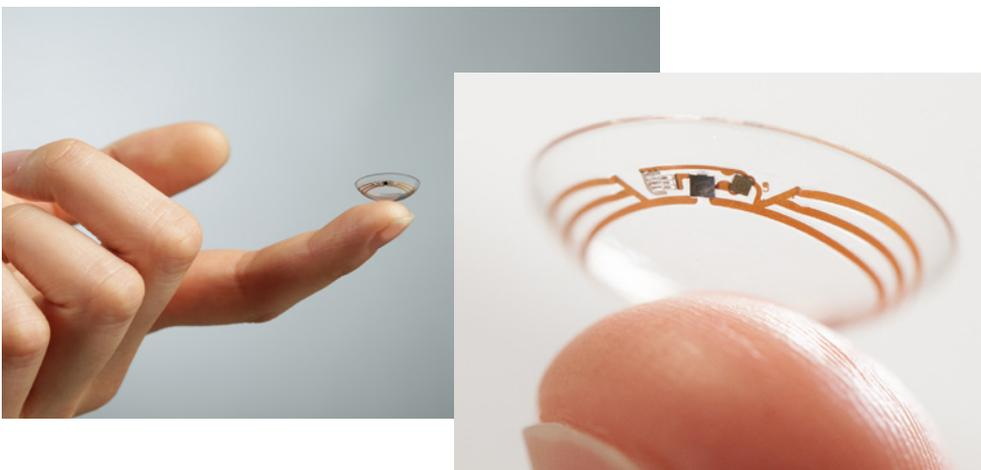
**Figure 11** Glucose-monitoring contact lenses
