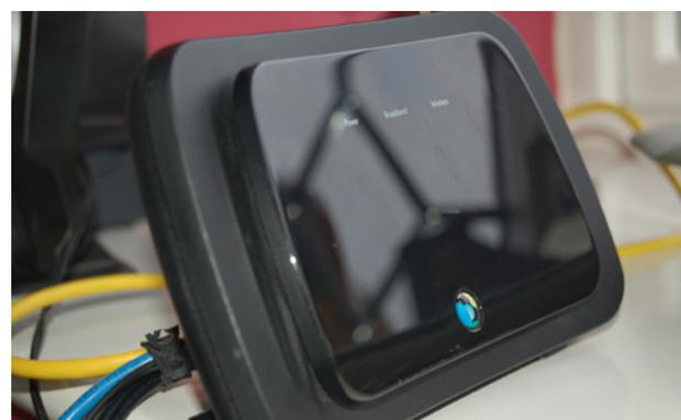
**Figure 2** A typical hub, which includes a router, Wi-Fi controller and wired network ports
