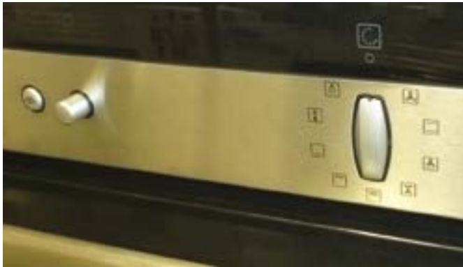
Buttons that stay pushed in or pop out to indicate on or off
