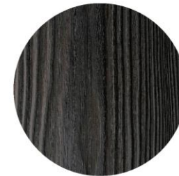
Charred timber cladding
