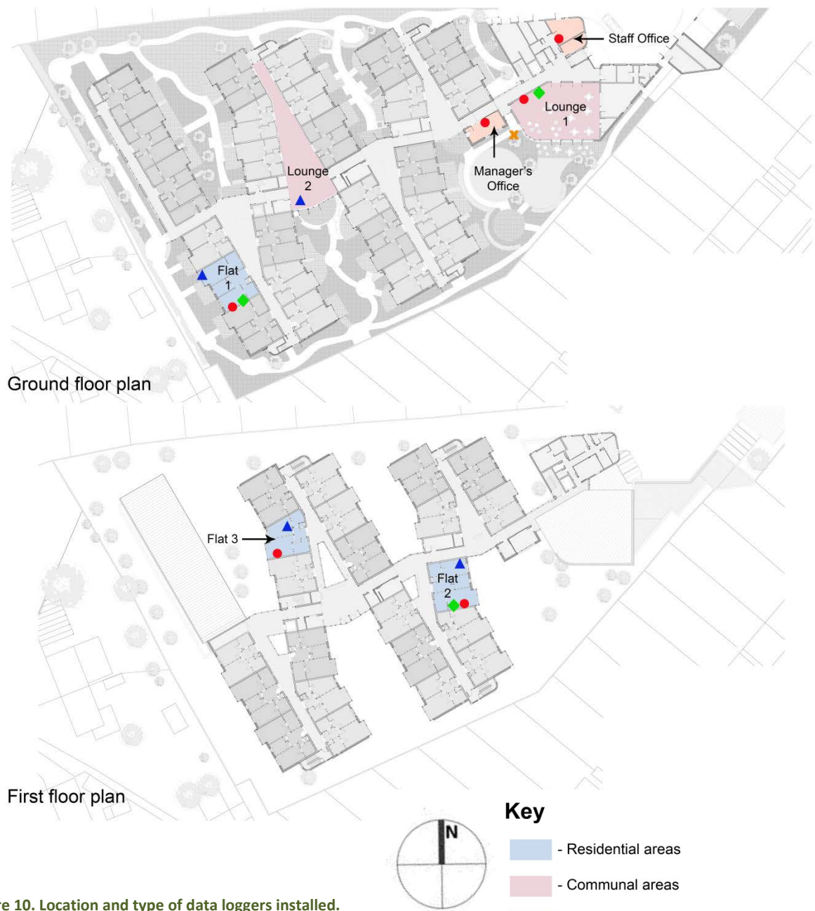
Figure 10. Location and type of data loggers installed.
