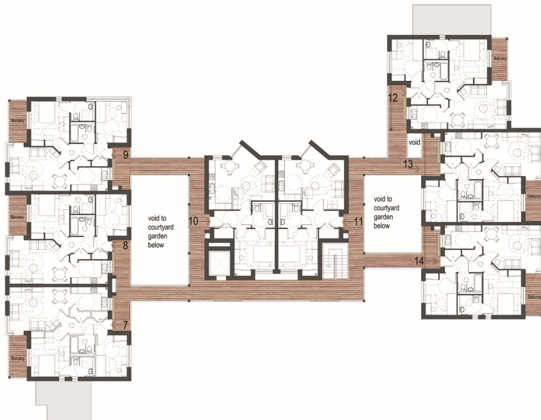
First Floor Plan showing arrangement of external walkways
