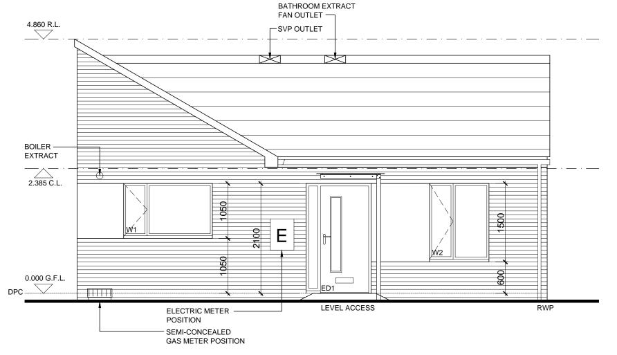
PROVIDE 1200MM LEVEL PLATFORM OUTSIDE FRONT DOOR COMBINED WITH A LEVEL, RAMPED OR STEPPED APPROACH ALL IN ACCORDANCE WITH APPROVED DOCUMENT M SECTION 6 -REFER TO SPECIFICATION FOR DIMENSIONAL CRITERIA.
