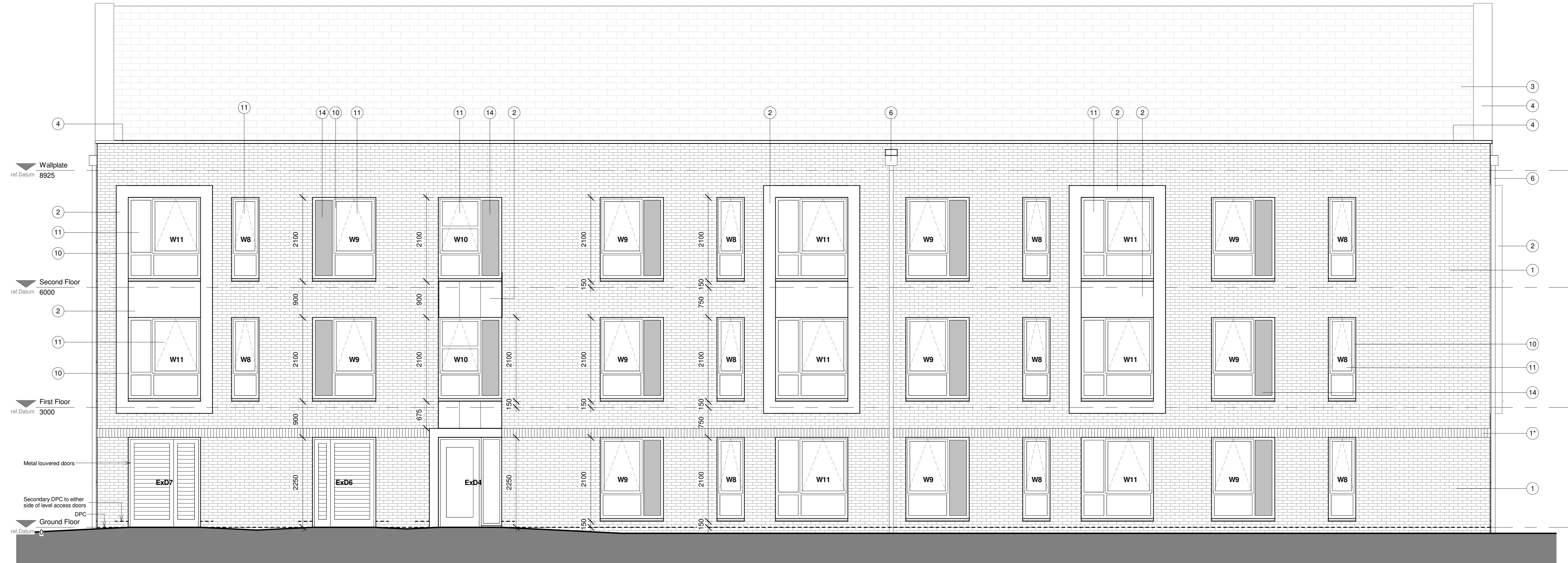
Rear Elevation onto courtyard parking 1 : 50
