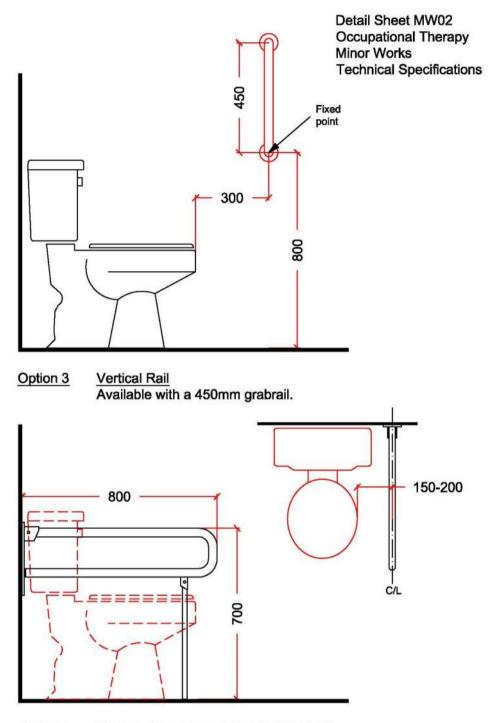
Option 4Folding down Hinge Supported grabrail<br/>To be fitted at 150-200mm from side of toilet.<br/>Note: This location may not always be<br/>possible due to obstructions (eg WHB etc).<br/>OT to specify distance from toilet (as shown) if<br/>standard fitting not feasible.
