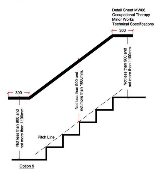
Internal Stairails Wooden rail with cylindrical grip, fitted similar height to existing handrail (see drawing). To continue on landings 300mm on the horizontal line, where technically feasible.
