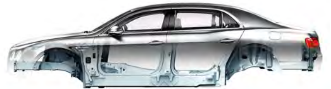
Platform Designing: The same 2018 underbody components in modified layout underpin both the Porsche Panamera (above) and Bentley Continental Flying Spur (bottom)
