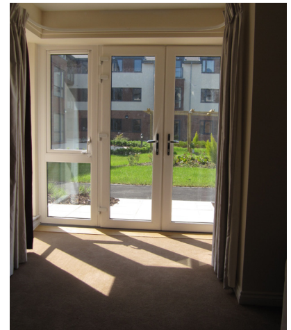
Single-aspect apartments are prone to poor daylighting, even where large areas of glazing are provided (image: Swallowdale Extra-care, Edlington).
