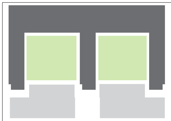
Figure / ground plan building footprint 4150 sq m site 12000 sq m site / footprint ratio 35% 75 dwellings/hectare
