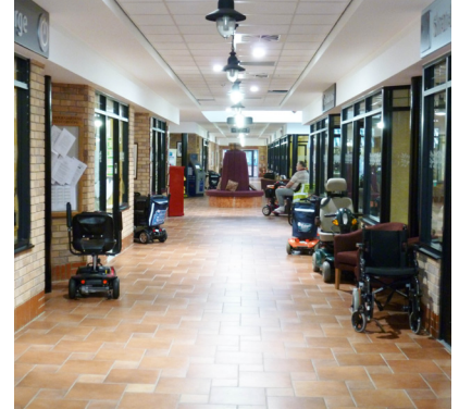
Semi-public communal areas can suffer from poor daylighting and a lack of space to stow mobility aids (image: Brunswick Gardens retirement village, Sheffield).
