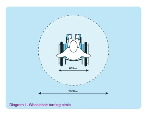
The overall width of a wheelchair is approximately 635mm when it is unoccupied. Additional space is needed at each side of the chair to enable the user to propel it manually.
