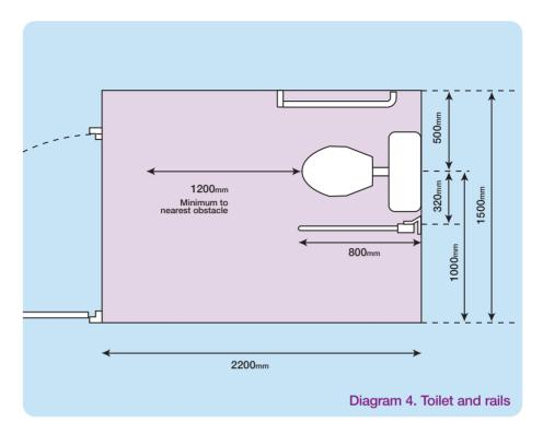
An S trap waste should be fitted as a P trap running 90 degrees to the toilet would prevent the fitting of a toilet frame and restrict wheelchair accessibility.
