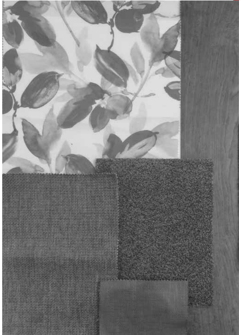
Monochrome image demonstrating comparative light reflectance value (LRV) of materials
