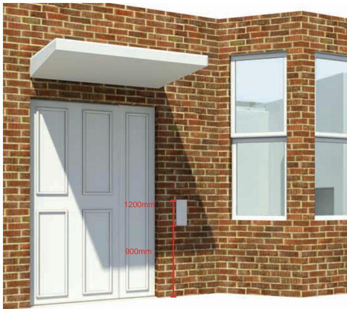
Figure 3.3 Dwelling entrance access control system
